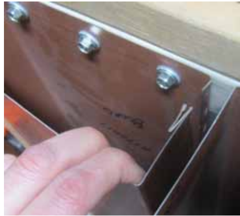
Photo No. 12 Specimen 172297 button lock separation after testing
