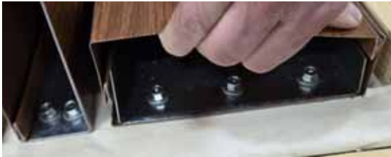
Photo No. 9 Specimen 172282 button lock separation after testing
