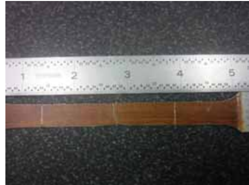
Photo No. 2 Specimen 173207 board after tensile test
