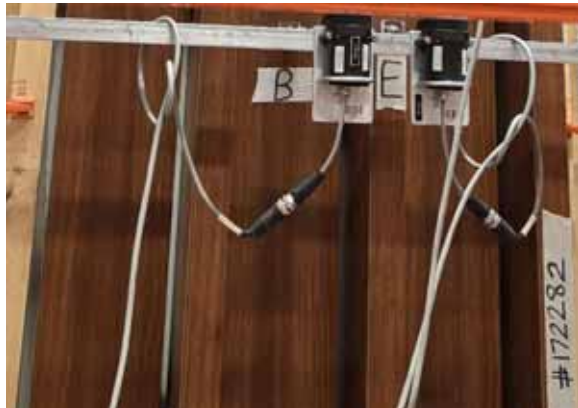
Photo No. 5 Specimen 172282 middle gauge labels and locations
