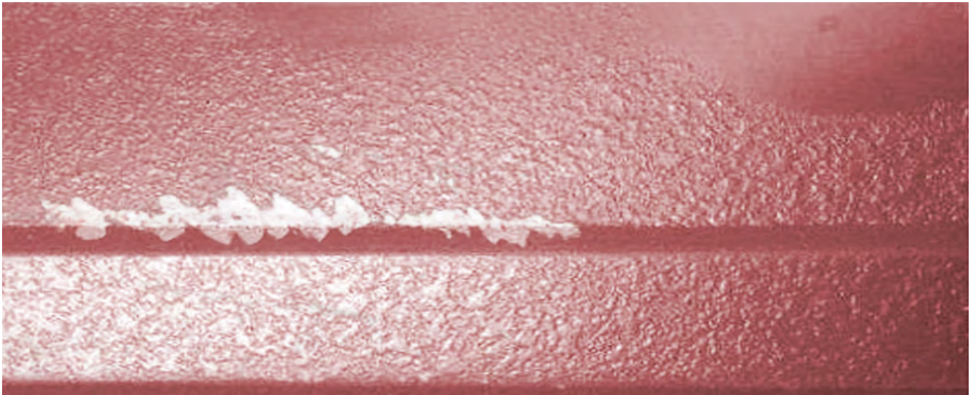
Close-up image of severe "Wet Stack Corrosion." Note smooth, normal surface in upper right corner. Note when scratched, the primer has been compromised as well as the presence of Zinc Oxide (white rust).
