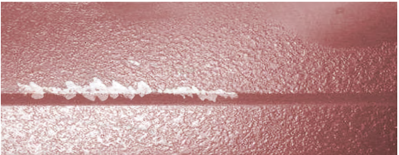
Close-up image of severe "Wet Stack Corrosion." Note smooth, normal surface in upper right corner. Note when scratched, the primer has been compromised as well as the presence of Zinc Oxide (white rust).
