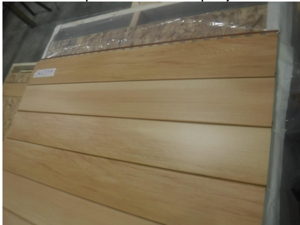
Photo No. 12 ASTM E330 – Specimen No. 163199 Completely Constructed (2)
