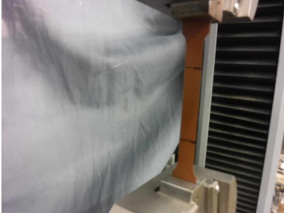
Photo No. 3 ASTM E8 Tensile Testing on Specimen No. 162819 (3)
