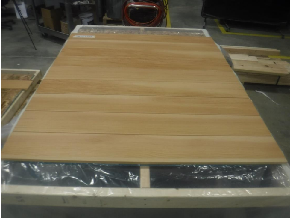
Photo No. 11 ASTM E330 – Specimen No. 163199 Completely Constructed
