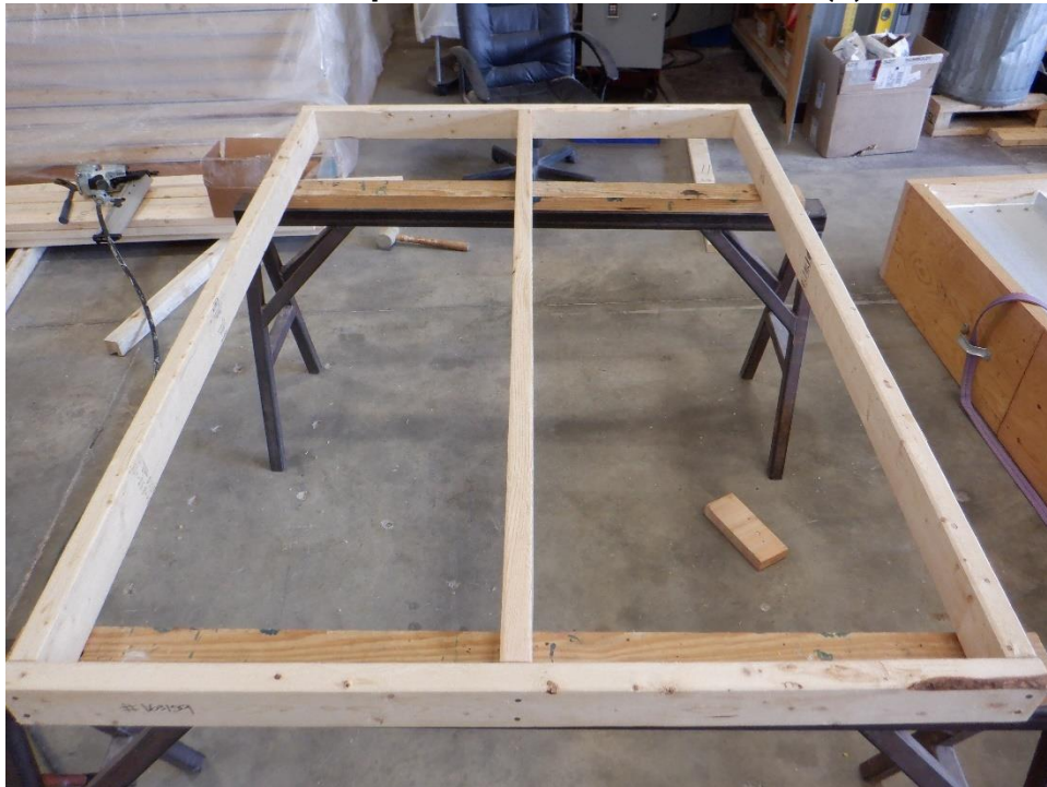
Photo No. 6 ASTM E330 Test Frame
