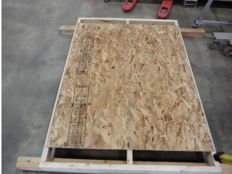
Photo No. 7 ASTM E330 Test Frame (2)
