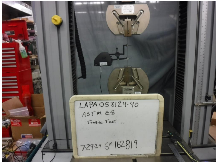
Photo No. 1 ASTM E8 Tensile Testing on Specimen No. 162819
