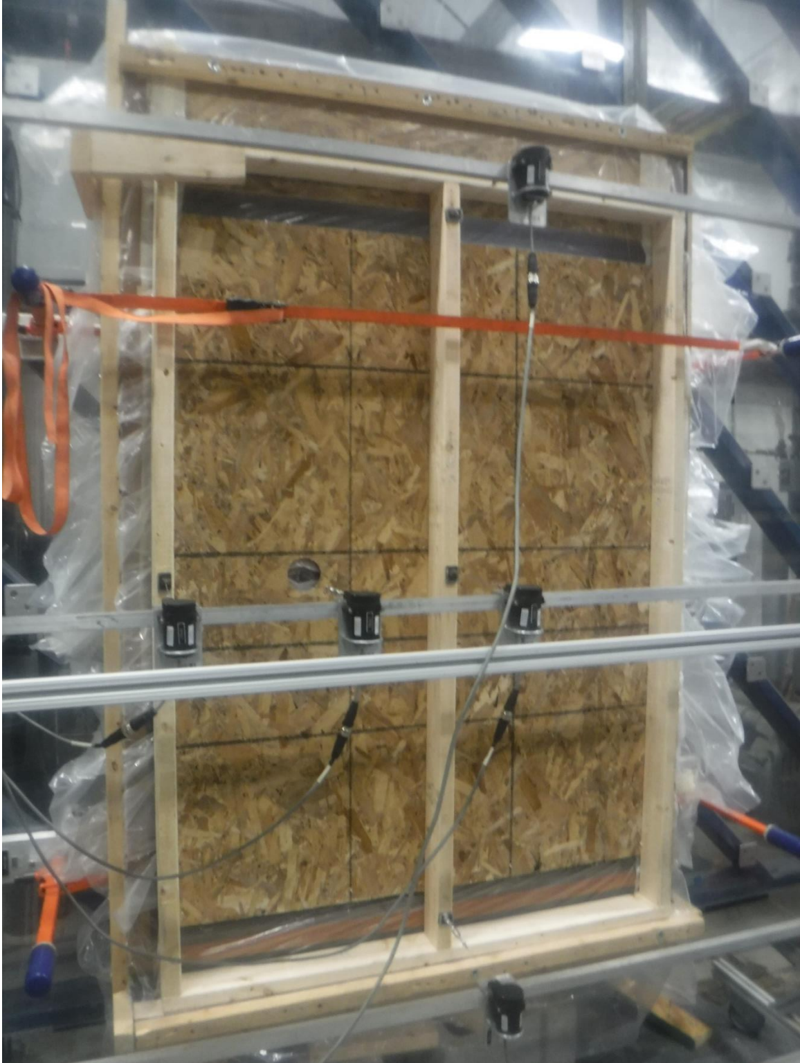
Photo No. 13 ASTM E330 – Specimen No. 163199 Attached to Test Wall
