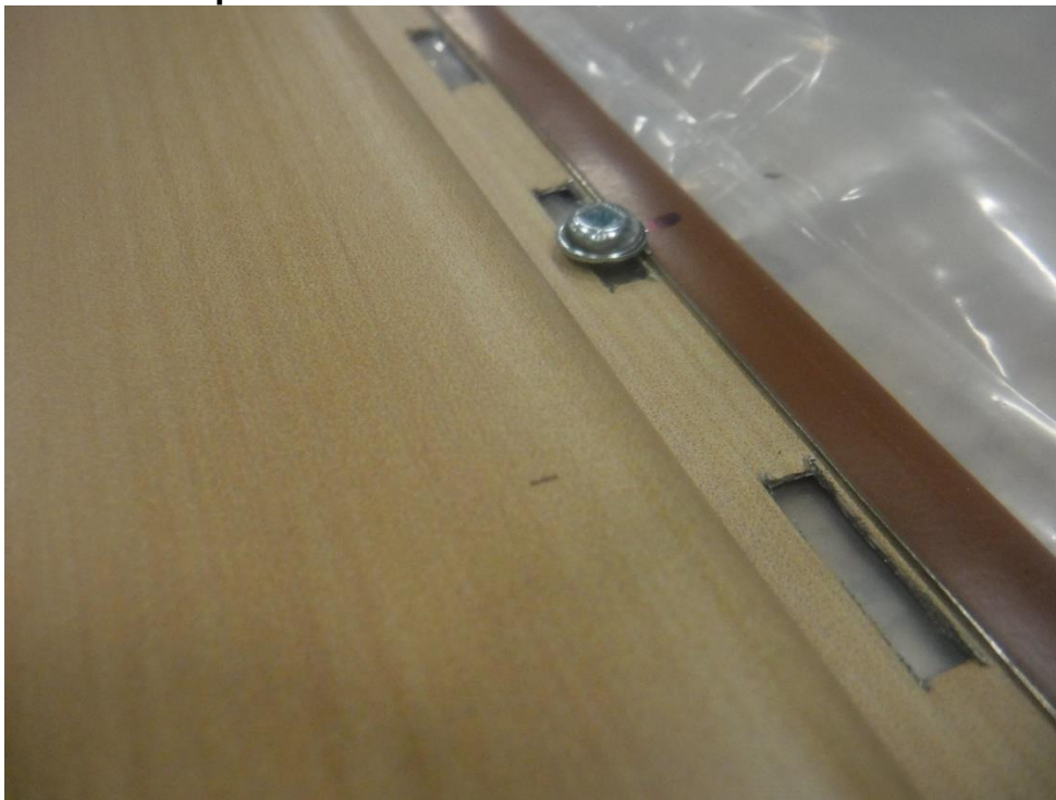
Photo No. 10 Specimen No. 163199 - 24-in. o.c. Fastener (2)
