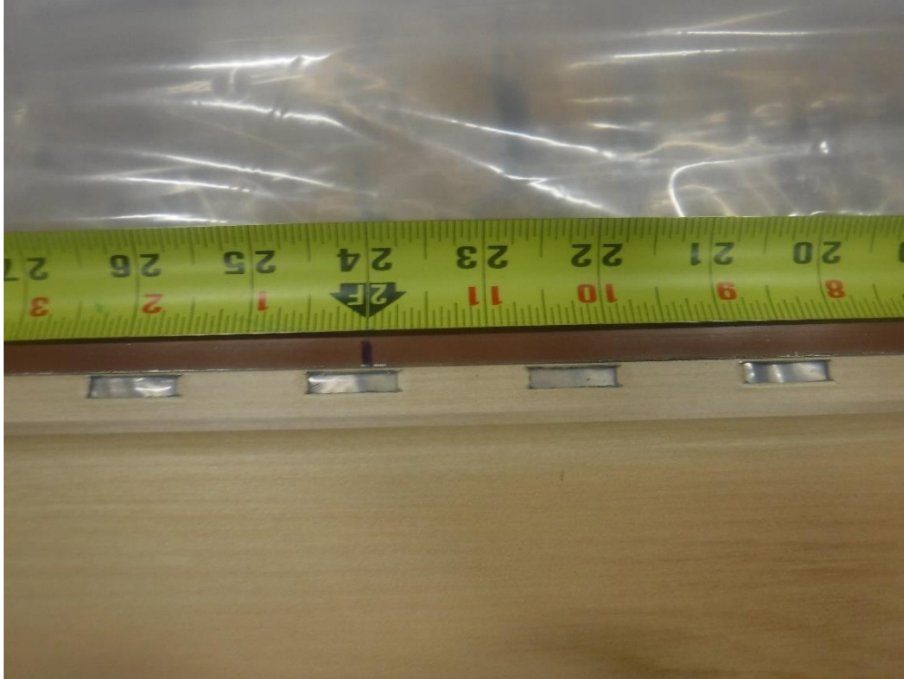
Photo No. 9 Specimen No. 163199 - 24-in. o.c. Fastener
