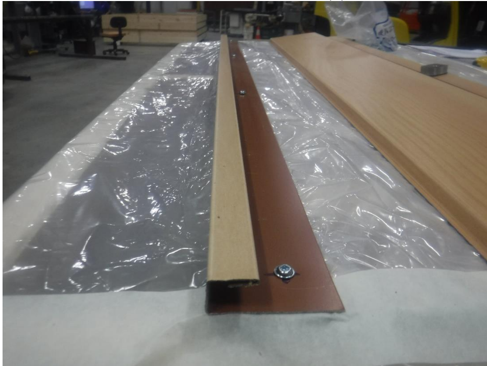
Photo No. 8 ASTM E330 - Starter Strip on Specimen No. 163199
