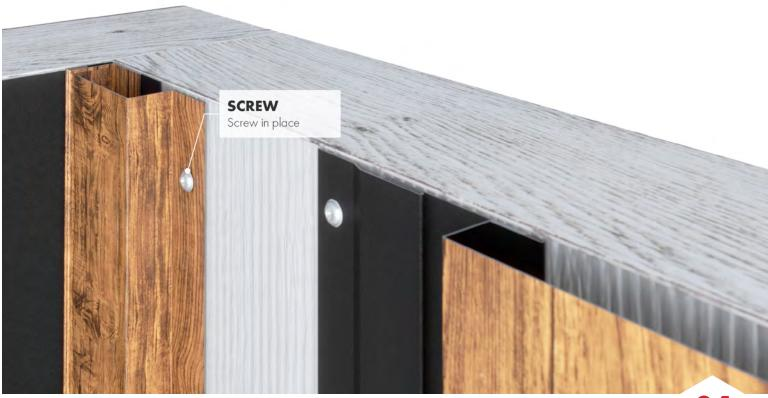
• The next step is to measure, cut, and attach the Z-Support. This trim is used as supplementary support for the Random Plank, as you will need to trim the Random Plank edge to ensure it cleanly ends in the corner. Push the Z-Support firmly against the Bottom J Receiver and fasten to the substrate.
