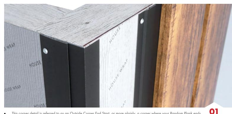
• This corner detail is referred to as an Outside Corner End Start, or more plainly, a corner where your Random Plank ends and starts in two different directions a 90-degree angle. To begin your Outside Corner End Start Corner, measure & cut one Outside Corner Starter Strip to length for your project. The OS Corner Starter Strip is reversible, so place the longer side on the wall where you want your 1" reveal to show. Attach to substrate with the appropriate wood or metal screws.
