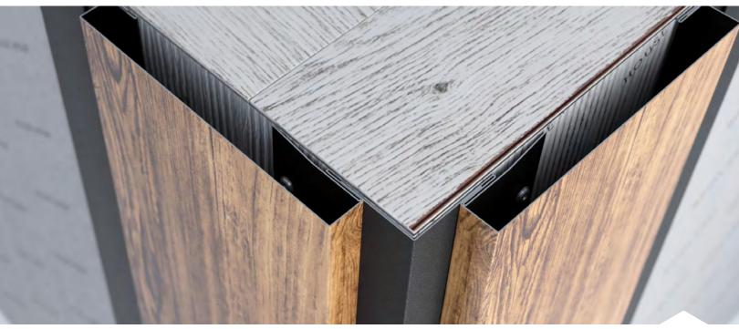
• Next, slide your Joiner Trims behind your chosen Random Planks. Gently pull the joiner so it is sitting flush along the length of the Random Plank. Then fasten the Joiner Trim between the hems with the appropriate screws.
