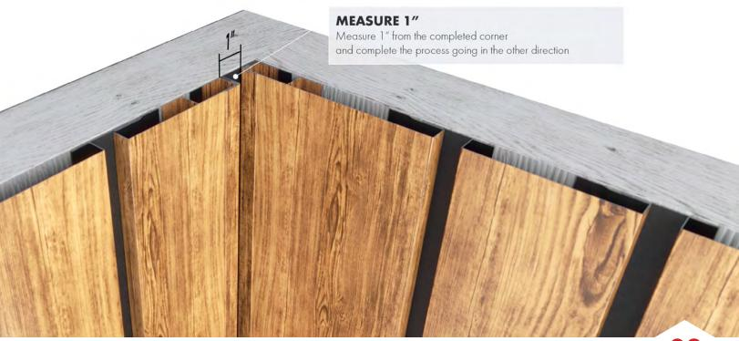
To complete the other side of the Inside End End corner, repeat these steps starting from the other direction. Leave a 1" inch
