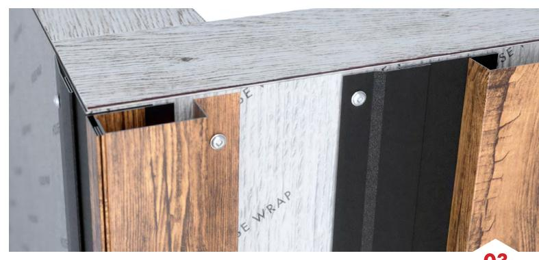
• The next step is to measure, cut, and attach the Z-Support. This trim is used as a supplementary support for the Random Plank as you will need to trim the Random Plank edge to ensure it cleanly ends in the corner. Push the Z-Support firmly against the Bottom J Receiver and fasten to the wall.
