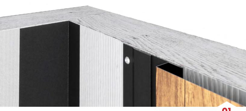
• This corner detail is referred to as an Inside End Start corner, or more plainly, a corner where your Random Plank ends and you need to start again in another direction. To begin your End Start corner, measure & cut an Inside L-Trim to fit. The L-Trim is reversible, so place the longer side on the wall where you want your 1" reveal to show. You do not have to attach the L-Trim yet as you will be placing another trim section overtop of the L-Trim.
