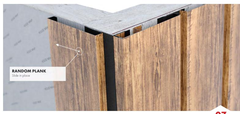
• After the End is installed, you can start in the other direction. To begin, slide your first Random Plank into place. In this case, you will pull or push the Random Plank snug against the inside of your Outside Corner Starter Strip.
