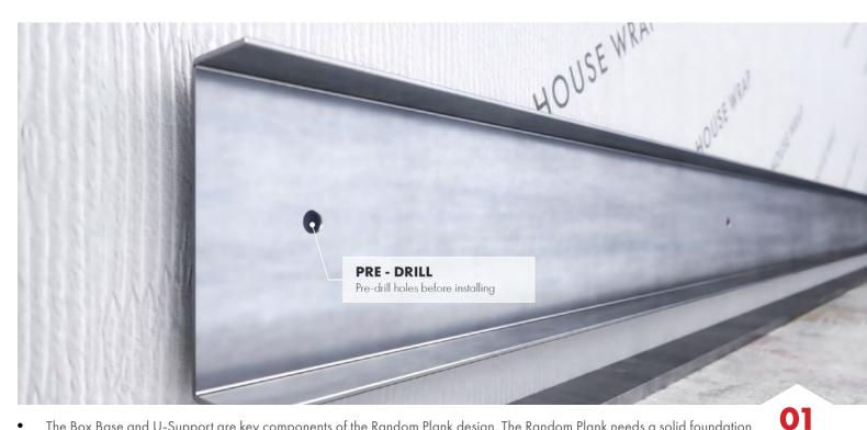
• The Box Base and U-Support are key components of the Random Plank design. The Random Plank needs a solid foundation to ensure there is no distortion or sliding of the panel. The U-Support is made from heavier gauge steel. Screw holes should be pre-drilled and aligned with substrate studs.
