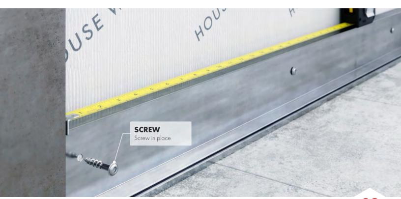
• To install the Box Base, start by measuring the U-Support to fit the length of your wall. It can be cut to measure following one of the outlined methods at the beginning of this guide, and can also be set side-by-side to extend a longer wall. Before installing the U-Support, pre-drill your screw holes (no farther than 30" apart) as this is very thick steel. Attach the U-Support 1/4" from the ground or bottom level. Screw in place using appropriate fasteners for wood or steel.
