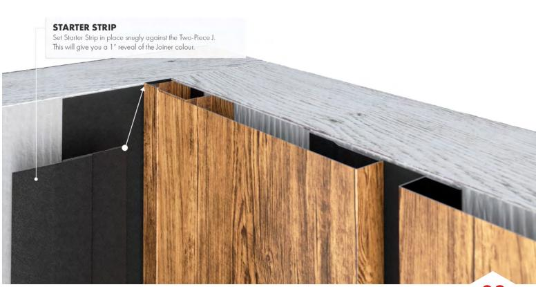
• This image shows the already measured & cut Starter Strip sliding into place. Ensure your Starter Strip is aligned with the top of your Two-Piece J-Channel. Once aligned, the Starter Strip can be fastened to the substrate through the angled flange using the appropriate wood or metal screws.
