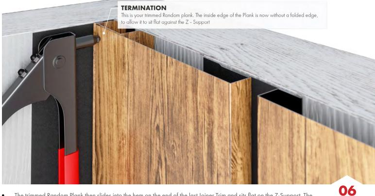
The trimmed Random Plank then slides into the hem on the end of the last Joiner Trim and sits flat on the Z-Support. The Random Plank is then fastened using Stainless Steel Rivets.
