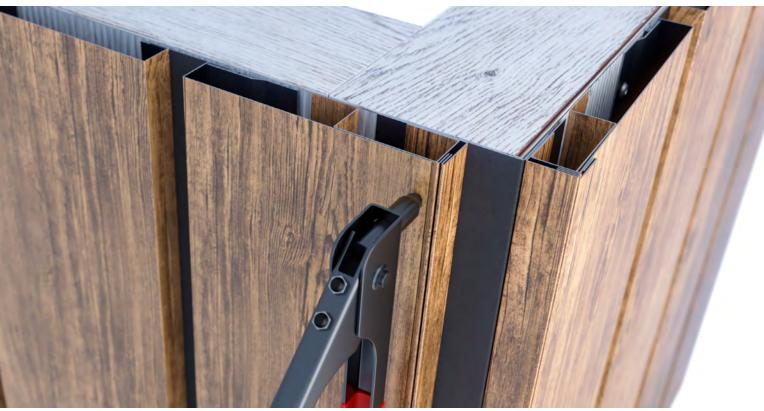
• The trimmed Random Plank then slides into the hem on the end of the last Joiner Trim and sits flat on the Z-Support. The Random Plank is then fastened using stainless steel rivets.
