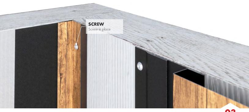
Push firmly on the Bottom J Receiver and the L-Trim to make sure they are snugly in place in the corner. Next, fasten both
