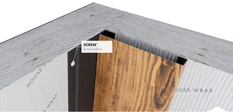
Push firmly on the Inside Corner Starter Strip and the Random Plank to make sure they are snugly in place in the corner. Next, fasten the Inside Corner Starter Strip to the substrate with the appropriate wood or metal screws. Ensure you screw through the slanted flange and not through the hem where the Random Plank needs to slide into.
