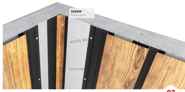
• Push firmly on the bottom J Receiver and the L-Trim to ensure that they are snugly in place in the corner. Fasten both trims to the substrate with the appropriate wood or metal screws. Ensure you screw through both layers of the bottom J and the L-Trim. The maximum distance you should have between screws is 30".
