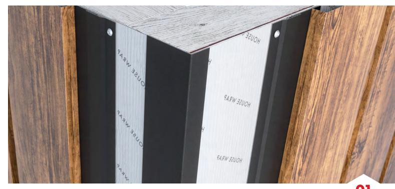
• This corner detail is referred to as an Outside End End corner, or more plainly, a corner where your Random Plank ends from both directions. To begin your End End corner, measure and cut an Outside L-Trim to the height of your wall. The L-Trim is reversible, so place the longer side on the wall where you want your 1" reveal to show. You do not have to attach the trim yet as you will be placing another trim section overtop of the L-Trim.
