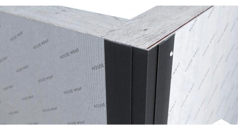
Take the second trimmed OS Starter Strip and flip it around. The trims are designed to be long enough to just slip into the other trim's joiner hem. Slide the second OS Starter Strip into the first and press firmly against the corner substrate. Next, fasten the second Outside Corner Starter Strip to the substrate with the appropriate wood or metal screws.
