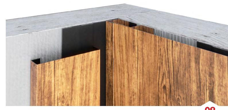
• Once your Starter Strip is installed, slide your first Random Plank into place. In this case, you will pull or push the Random Plank snug against the inside of your Starter Strip.
