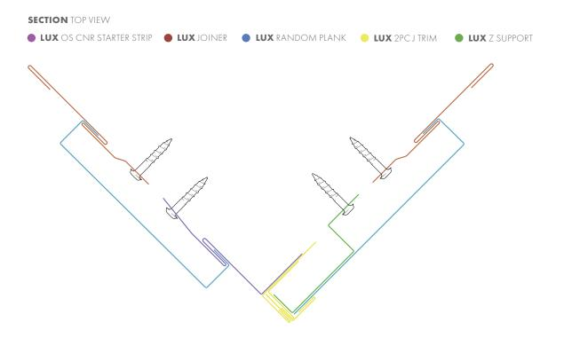
• This illustration of the top view demonstrates how the trims and Random Planks should be joined together.
