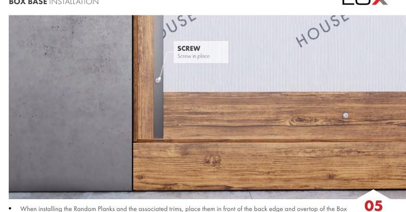
When installing the Random Planks and the associated trims, place them in front of the back edge and overtop of the Box Base. Here we have a J-Trim installed over the Box Base.
