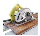
LUX Planks can be cut using metalworking snips, metalworking nibblers, or various power saws. A metal cutting blade such as Freud Diablo Steel Demon 48 tooth TCG Ferrous Metal Cutting Blade is recommended.
