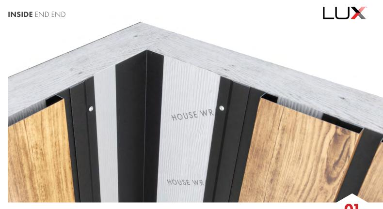
This corner detail is referred to as an Inside End End corner, or more plainly, a corner where your Random Plank project ends from both directions. To start your Inside End End corner, measure & cut an Inside L-Trim to fit the height of your wall. The L-Trim is reversible, so place the longer side on the wall where you want your 1" reveal to show. You do not have to attach the trim yet as you will be placing another trim section overtop of the L-Trim.
