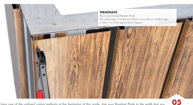
Using one of the outlined cutting methods at the beginning of this guide, trim your Random Plank to the width that you measured in the previous step. The trimmed Random Plank then slides into the hem on the end of the last Joiner Trim and sits flat against the Z-Support. The Random Plank is then fastened using stainless steel rivets.
