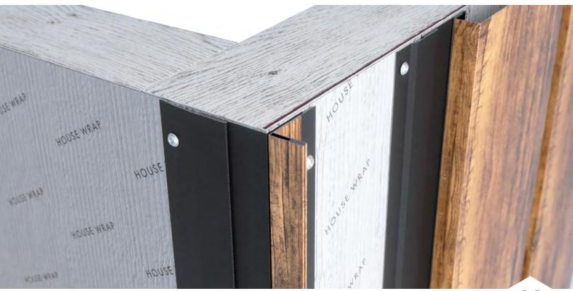
• Next, measure the distance your Two-Piece J-Channel needs to be from end to end to fit the height of the wall. You can cut the J using one of the methods in the cut guide shown at the beginning of this guide. Once the Two-Piece J is cut, slide the Top J Insert out of the Bottom J Receiver and place in front of the Outside L-Trim. Next, fasten both trims to the substrate with the appropriate wood or metal screws. Ensure you screw through both layers of the Bottom J Receiver and the L-Trim.
