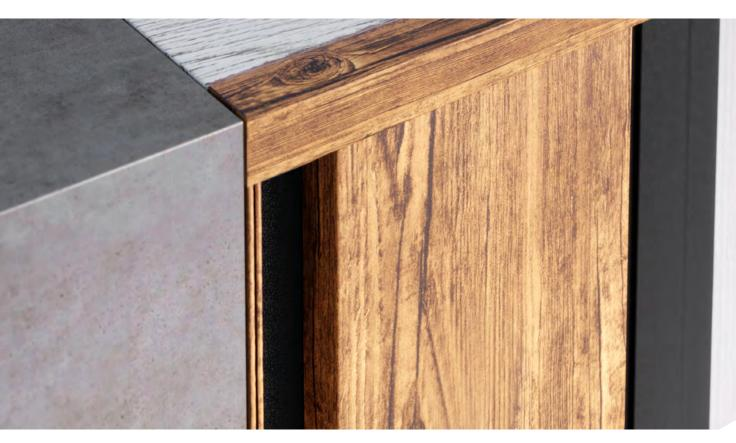
• The Joiner Trim is designed to be slid underneath the Random Plank, then pulled back until it catches the hem on the inside of the Random Plank. Gently pull the Joiner Trim so that it is sitting flush along the length of the Random Plank. You can then fasten the Joiner Trim between the hems with the appropriate screws. Ensure not to screw through the hem that the next Random Plank needs to sit in. Otherwise, it will not fit.
