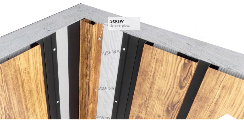
• The next step is to measure, cut, and attach the Z-Support. This trim is used as supplementary support for the Random Plank, as you will need to trim the Random Plank edge to ensure that it sits tightly in the corner. Push the Z-Support firmly against the bottom J receiver and fasten to the wall.
